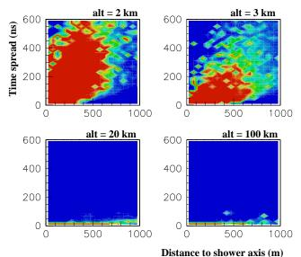
Fig. 2. Particle time spread with respect to a planar shower front versus distance to the shower axis for  $10^{19}$ eV protons at 80 deg zenith angle. The primary altitude is given at the interaction point, early interactions (bottom) correspond to high altitude and produce old shower at the ground level, late interactions (top) correspond to penetrating particle and young shower.
